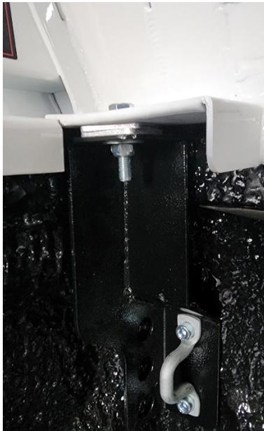
Pic 15 – Front mounting bracket In position and tightened
