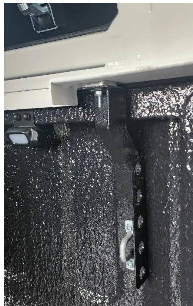
Pic 16 – Rear mounting bracket in position and tightened.
